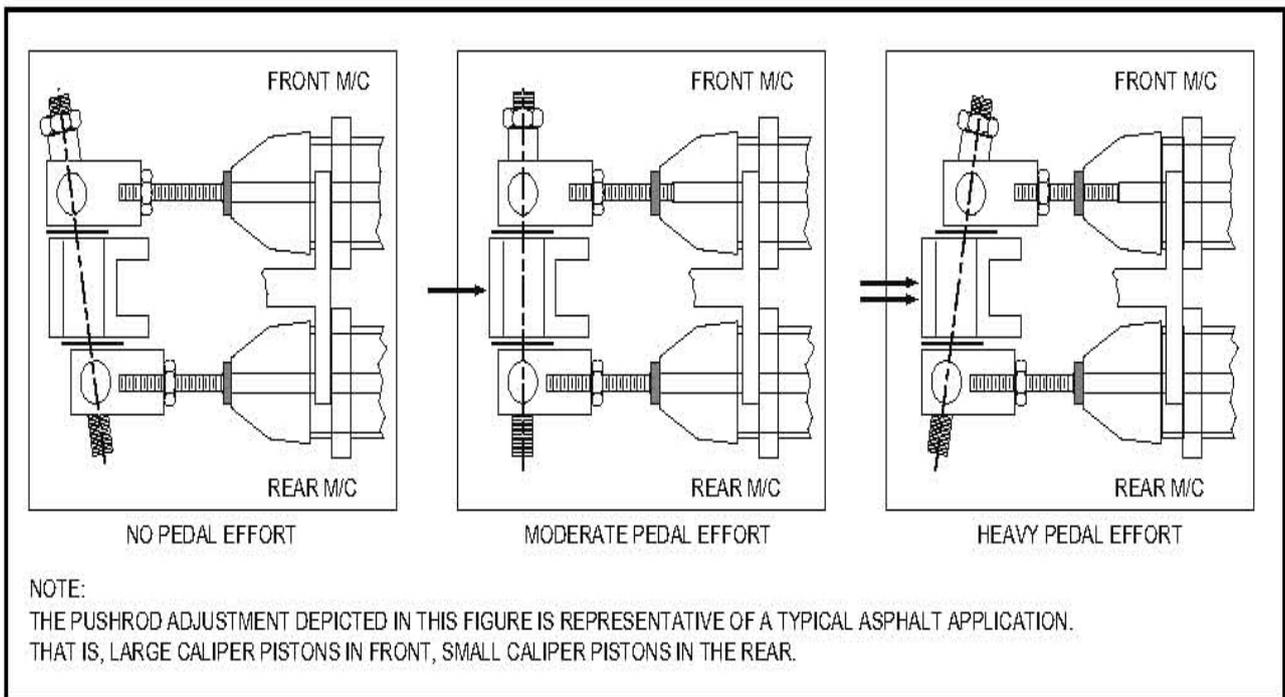
**Figure 2. Balance bar lever adjustment**
