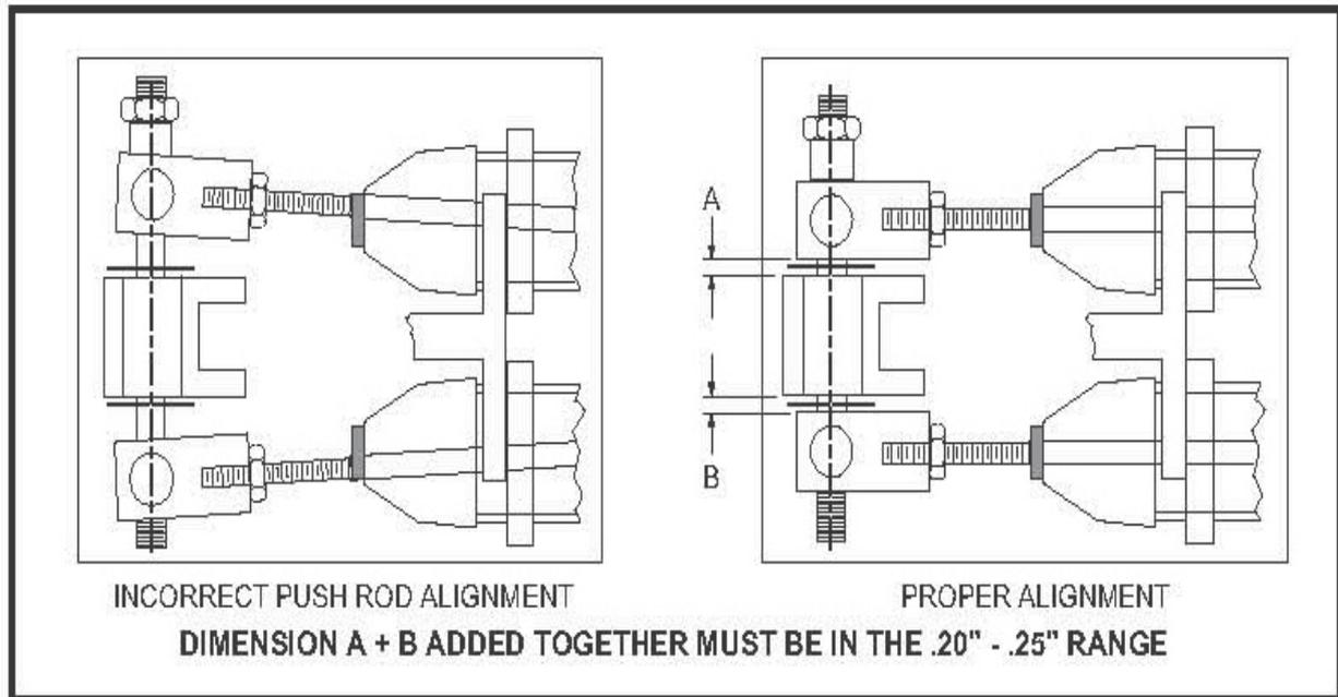
Figure 4. Example of pushrod alignment
