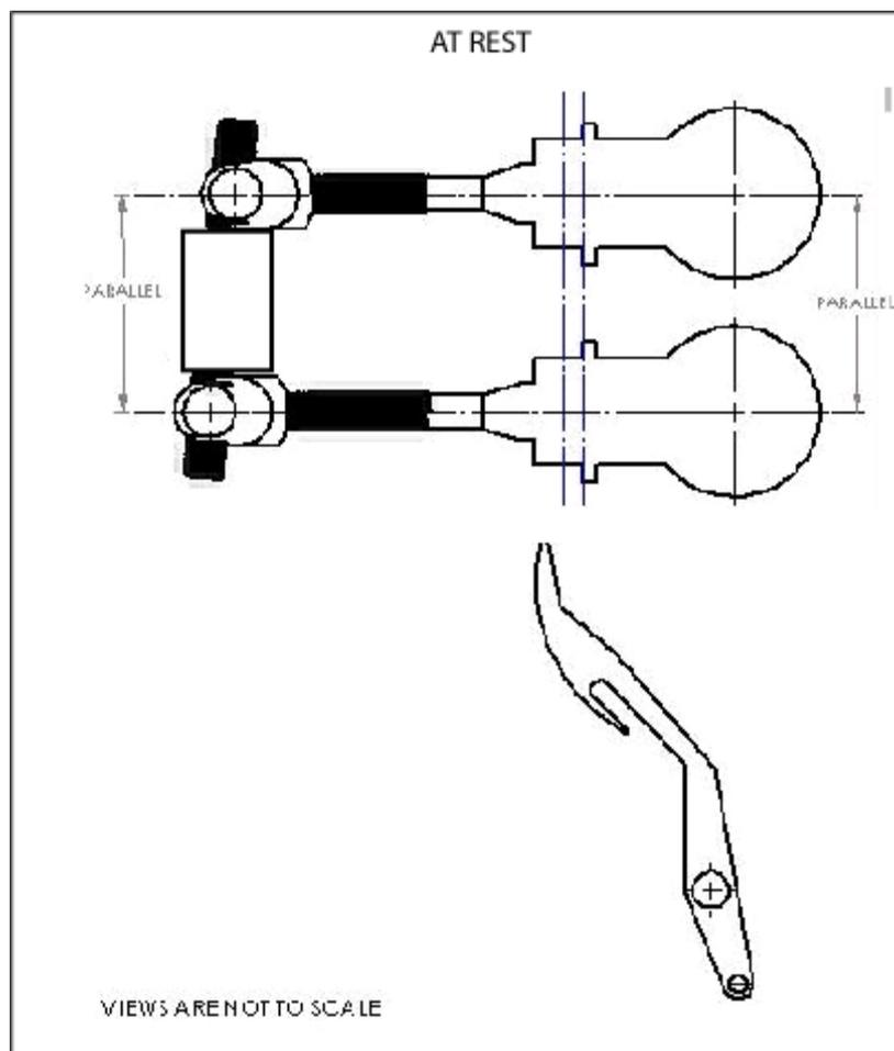
First, we must insure that the bias bar pivot bearing is free to move within the pedal tube. Often this tube becomes distorted during installation. If this is the case, then the tube may be honed, until the bearing slides smoothly from one end of the tube to the other. The tube must be clean, and may be lubricated with a light oil or dry Teflon spray.
