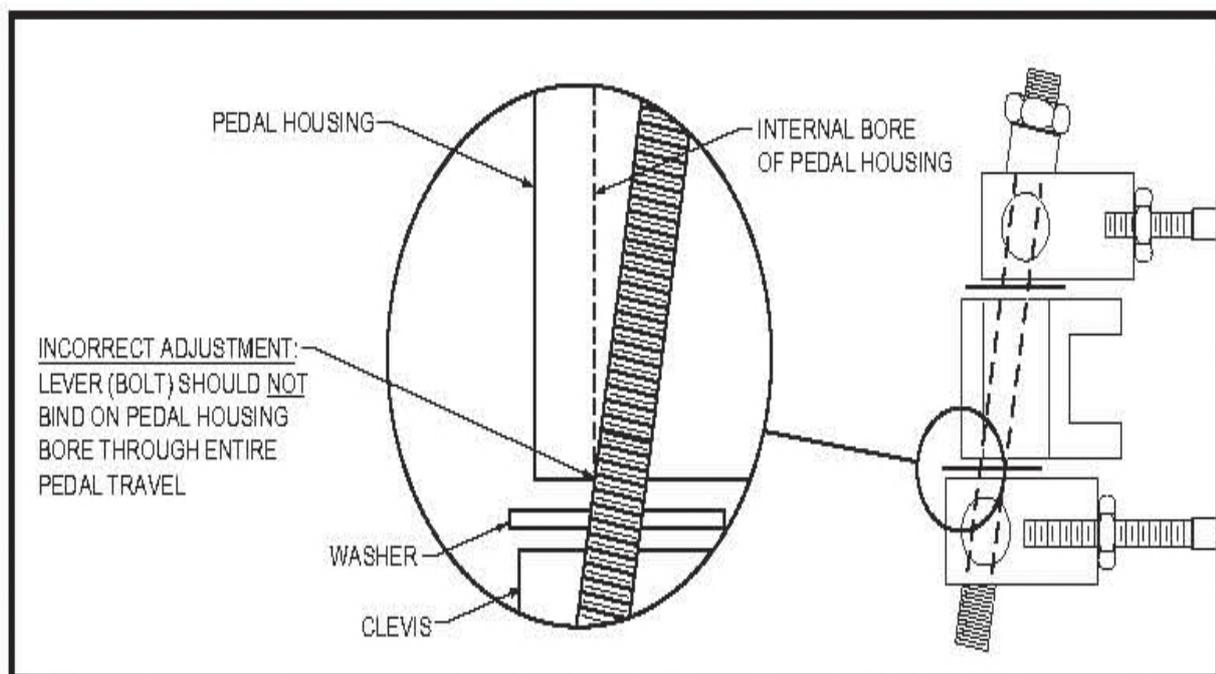
Figure 3. Balance bar lever interference
