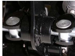
Balance bar giving you total control over the front to rear braking.
