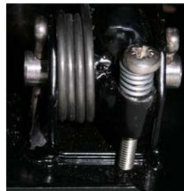
Adjustable spring loaded accelerator pedal. Allowing the pedal to be positioned exactly to your requirements.
