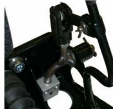
Light weight accelerator linkage included. Will accept single or twin cables.
