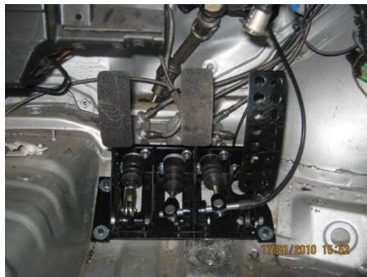
When bolting the pedal box in make sure you use high tensile bolts and large washers to spread the load when the brake is applied, never use riv-nuts or similar fixings to mount a pedal box!!!
